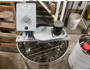
10. To operate extractor, turn knob to left (lowest speed). Then, turn the switch on to the "1" position. Gradually increase speed until the extractor spins.
