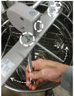
3. Temporarily place the motor on the top bar as shown below. There are two bolts that will align with holes in the top bar. Do not install the nuts yet.
