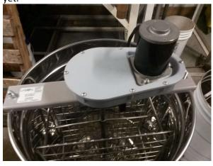
**Note:** for 12-frame models, you may need to move the hinges on the right side to the right to make room for the motor. Re-attach the hinges with ½ of the screws (see below).
